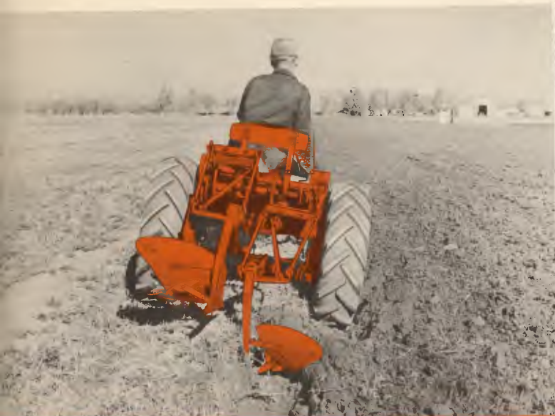
No dead furrows and a level seedbed with two-way mounted plow
