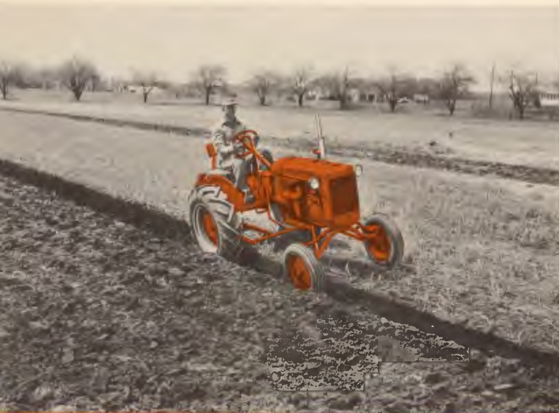
Plowing a deep seedbed with mounted moldboard plow
