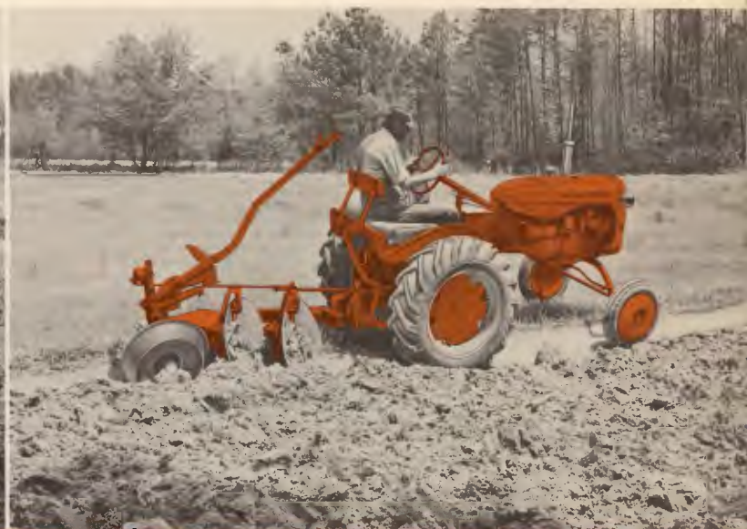
Preparing seedbed with semi-mounted disc plow
