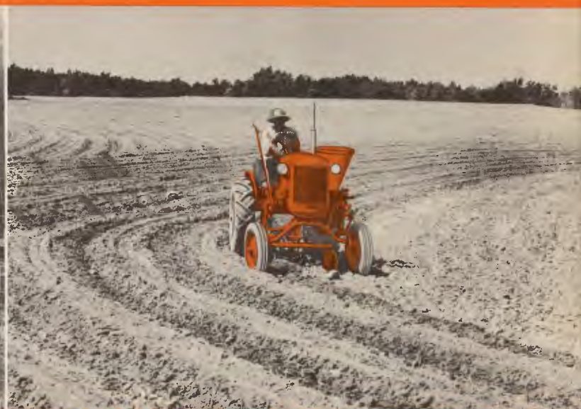
Planting cotton on the contour with front-mounted planter
