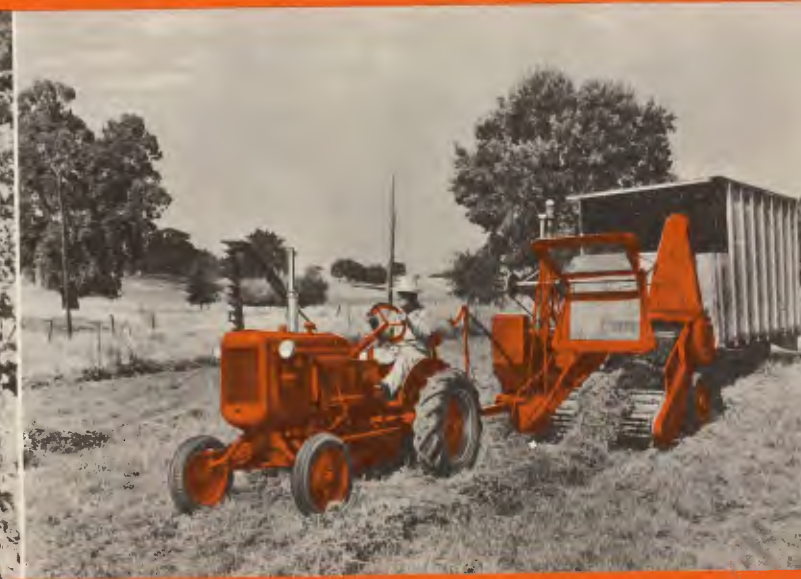
B and forage harvester with auxiliary motor making silage
